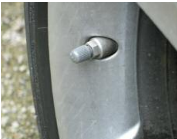
“Threaded” Valve Stem on Vehicles, which Monitor Actual Tire Pressure.
