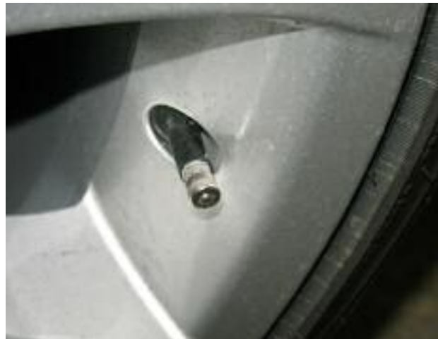
“Rubber” Valve Stem on Vehicles, which Monitor Wheel Speed.
