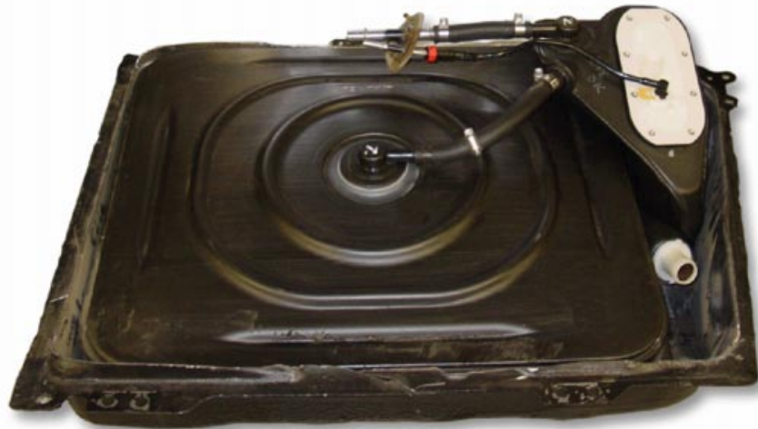
Tank cut opened to show bladder
