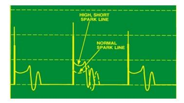
This is often caused by a sticking or worn valve in one cylinder that causes an uneven air/fuel ratio:
