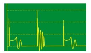
High secondary resistance in one or both plug cables High secondary resistance in the coil Corroded terminals at the coil or the cables, Very wide plug gaps:
