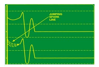
Usually indicates sticking or floating valves if it appears at all speeds. It also can indicate burned valves, wide plug gaps or a vacuum leak that affects several cylinders:
