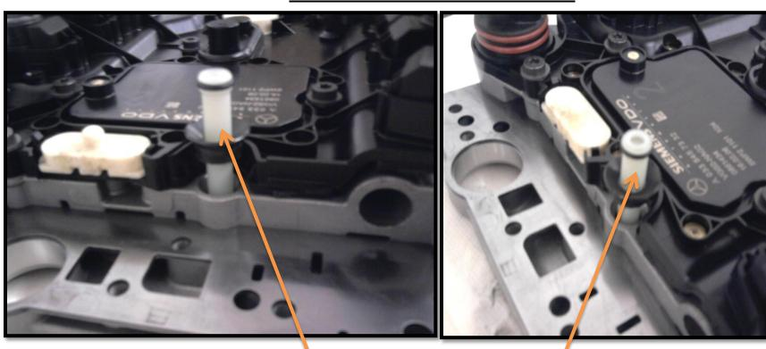
When replacing the valve body on the 722.9 gearbox remember to remove the white oil feed pipe from the shown location, and fit as next page suggests.
