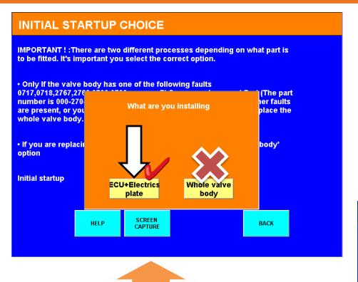
Choose between installing a complete valve body or just the **ECU and electrics plate**.
