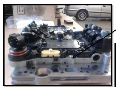
Oil filler pipe needs swapping over when fitting new valve body.
