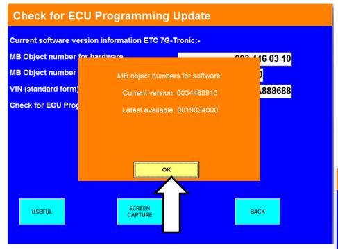
Remember a stable voltage is required Whilst flashing and SCN coding the control unit (failure to have stable voltage could result in failure and possible rendering the control unit un serviceable.
